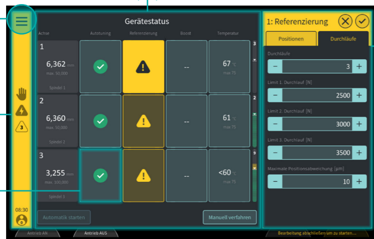
Main window with information on device status, axis positions, motion segments, etc.
