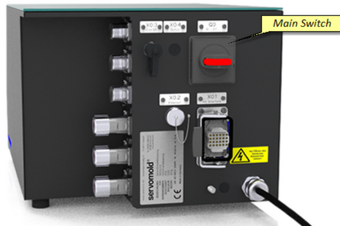
Fig. 3 Work station main switch on the Device (Servo Control System)
